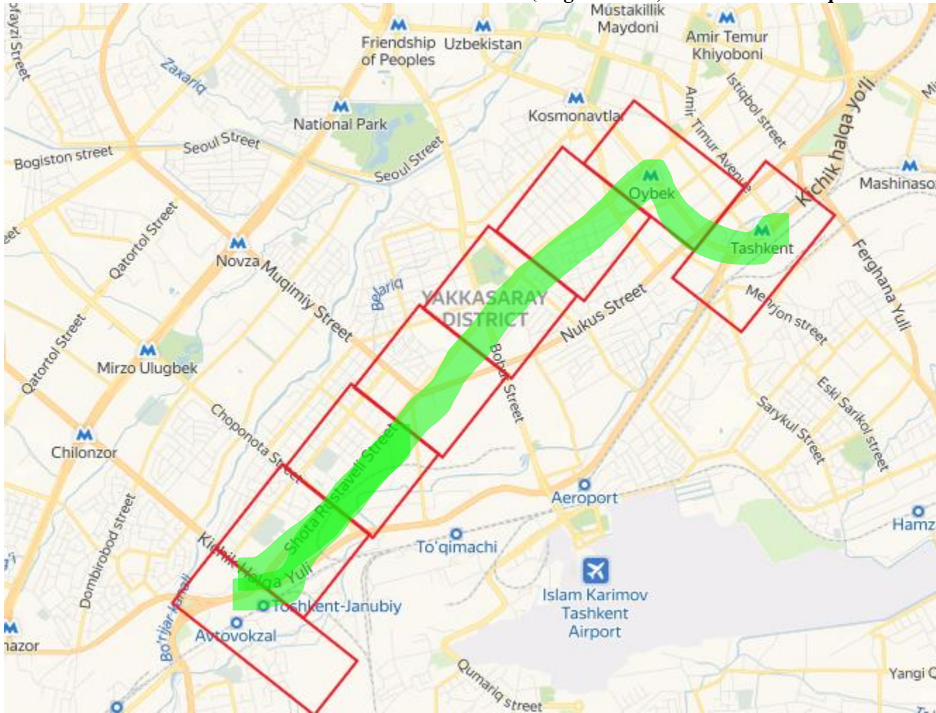
Figure 1-2: Assumed 1 km 2 areas around the Shota Rustaveli GUTC (length 7.5 km) to calculate consequential beneficiaries 49
